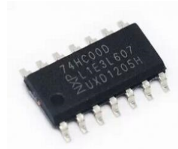
Figure 2.2.4: 74HC00 chip physical view
