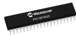
Figure 3.1.7: A PIC microcontroller. (Source: Microchip )
